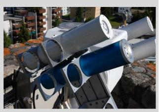
The Precision Filter Radiometer (PFR) is a research grade instrument to measure direct solar irradiance in 4 narrow spectral bands centered at wavelengths recommended by World Meteorological Organization for the determination of atmospheric aerosol optical depth (AOD).
