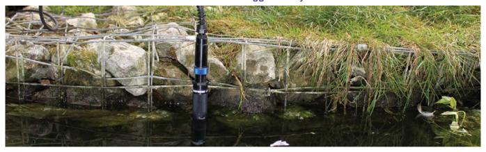
The AP-LITE is commonly used with our sapphire lensed turbidity sensor, chlorophyll sensor or blue-green algae sensors. Whilst the package includes an Aquameter the AP-LITE can also be used with one of our AquaLoggers for unmanned turbidity, chlorophyll or blue-green algae monitoring.
